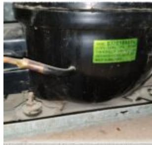
The Matsushita D77C18RAX5 is a legendary 1/4 HP refrigerator compressor optimized for R134a refrigerant. Known for its robust RSIR motor and 7.7cc displacement, it delivers 195W of cooling power for domestic freezers and refrigerators. This guide provides full technical data, wiring details, and the best professional cross-reference replacements for modern refrigeration repair.
