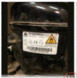
The Huayi HYB60MGU is a high-efficiency hermetic reciprocating compressor specifically engineered for Low Back Pressure (LBP) applications. Operating on the eco-friendly R600a refrigerant, this 1/7 HP unit is a primary component in modern household refrigerators. This guide provides an in-depth technical analysis, electrical wiring configurations, and reliable replacement alternatives for field engineers.
