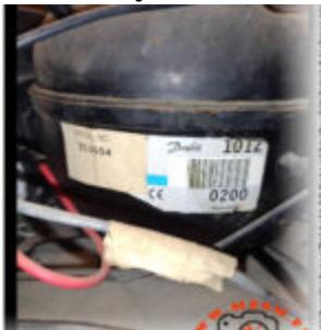
The Danfoss Secop BD35F 101Z0200 is the industry standard for DC mobile refrigeration. Engineered for 12V and 24V systems using R134a, this compressor offers variable speed performance from 1/8 to 1/5 hp. This Mbsmpro technical guide explores its electronic control unit, wiring schemas, and cooling capacities for trucks, boats, and solar-powered appliances.
