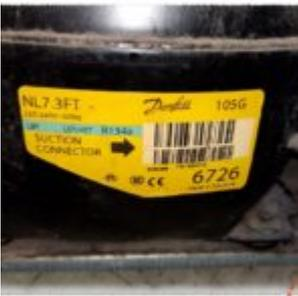
The Danfoss NL7.3FT is a cornerstone of domestic and light commercial refrigeration. Engineered for Low Back Pressure (LBP) applications using R134a refrigerant, this 1/4 HP unit offers reliability and high efficiency. In this guide, we break down the technical displacement, cooling capacity, and provide a comprehensive list of compatible replacements to ensure your cooling systems stay operational.
