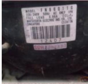
The Matsushita FN66Q11G is a highly reliable 1/6 hp reciprocating compressor designed for low back pressure applications. Operating on 220-240V at 50Hz, this R12-based unit was manufactured in Singapore and is known for its long-lasting performance in domestic refrigerators. Learn about its cooling capacity, amperage, and modern replacement options in this comprehensive technical guide.
