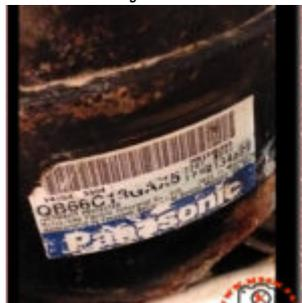
The Panasonic QB66C13GAX5 is a reliable 1/5 HP compressor designed for R134a LBP systems, commonly found in domestic refrigerators and freezers up to 250L capacity. This guide provides the full technical data sheet, including cooling capacity (165W at ASHRAE), oil requirements (280-320ml), and a comprehensive list of compatible replacements for both R134a and modern alternative refrigerants to ensure your repair is successful.
