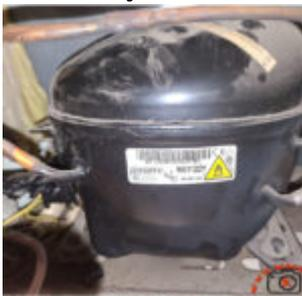
The Jiaxipera NX1122Y is a high-efficiency 1/4 HP compressor designed for modern R600a refrigeration systems. Commonly used in Whirlpool and Indesit appliances, it offers roughly 200W of cooling capacity at LBP conditions. This guide covers its full technical specifications, COP efficiency data, and provides a comprehensive list of compatible replacement models for technicians and DIY repair.
