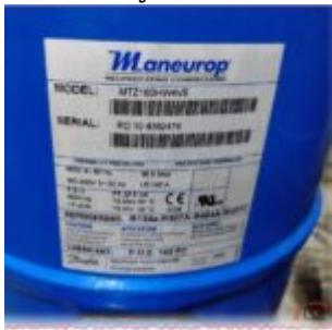
Maneurop MTZ160HW4VE 13 hp reciprocating compressor R404A R507A R134a R407C 20.3 kW medium temperature cold room applications
