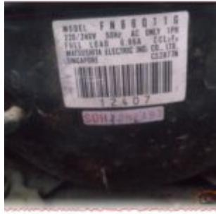
The Matsushita FN66Q11G is a highly reliable 1/6 hp reciprocating compressor designed for low back pressure applications. Operating on 220-240V at 50Hz, this R12-based unit was manufactured in Singapore and is known for its long-lasting performance in domestic refrigerators. Learn about its cooling capacity, amperage, and modern replacement options in this comprehensive technical guide.
