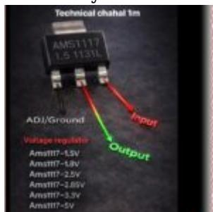
AMS1117 voltage regulator pinout input output ground fixed versions 1.5V 1.8V 2.5V 2.85V 3.3V 5V applications
