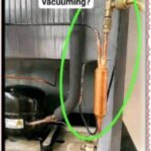
The copper tube assembly shown is a service charging valve on the liquid line of a small hermetic refrigeration unit. This single access point can be used for deep vacuum and for refrigerant charging, depending on the connected equipment. Understanding when the technician is vacuuming and when charging is critical for reliability.
