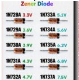
Zener diodes like the 1N4728A thru 1N4737A series deliver reliable voltage regulation from 3.3V to 7.5V at 1W power. Engineers rely on these for stabilizing circuits in power supplies and protection setups. Check the full voltage chart and specs below for your next project. (55 words)
