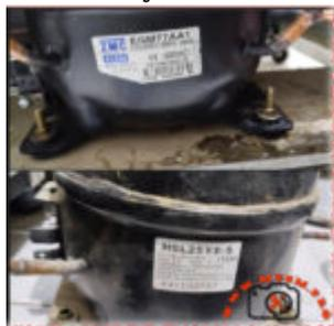
When a refrigerator stops cooling, the heart of the problem is often the compressor. Understanding the differences between the ZMC EGM77AA1 and the Daewoo HSL25YE-5 is vital for any technician. These R134a units are staples in the industry, offering reliable low back pressure performance for domestic and light commercial cooling systems worldwide.
