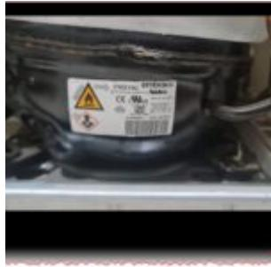
Mbsmpro.com, Compressor, FMXY9C, Embraco, R600a, 1/6 hp, Cooling, 220-240V, 1Ph 50Hz, LBP, Fullmotion, Inverter,  $-35^{\circ}\text{C}$  to  $-10^{\circ}\text{C}$ , CE UL, Austria
