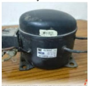
A 16 cubic feet Zanussi refrigerator typically relies on the GL90AA hermetic compressor, a compact piston unit built for R134a and low back pressure applications. This 1/4 HP motor offers cooling capacities from roughly 165 W up to around 346 W, giving enough reserve to maintain stable temperatures in family-size fridges even in hot kitchens.
