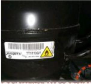
The Jiaxipera TT1113GY is a high-performance hermetic compressor engineered for Low Back Pressure applications using R600a (Isobutane). Featuring a 11.3 cm<sup>3</sup> displacement and a cooling capacity of 183 Watts, it represents the gold standard for modern energy-efficient refrigeration, offering exceptional reliability and reduced acoustic emissions in the domestic market.
