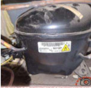
The Jiaxipera NX1122Y is a high-efficiency 1/4 HP compressor designed for modern R600a refrigeration systems. Commonly used in Whirlpool and Indesit appliances, it offers roughly 200W of cooling capacity at LBP conditions. This guide covers its full technical specifications, COP efficiency data, and provides a comprehensive list of compatible replacement models for technicians and DIY repair.
