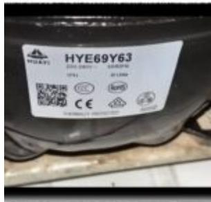
The Huayi HYE69Y63 is a highly efficient hermetic reciprocating compressor designed for low back pressure applications using R134a refrigerant. With a 1/5 HP rating and dual-frequency compatibility (50/60Hz), this motor is a cornerstone for domestic refrigerators and freezers. This comprehensive guide covers technical datasheets, electrical wiring, and professional replacement strategies for global cooling systems.
