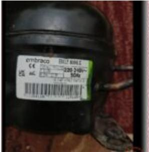
The Embraco EM2Z 80HL.C is a robust hermetic reciprocating compressor engineered for refrigeration efficiency. Featuring a 1/4 HP motor and optimized for R134a refrigerant, this Brazilian-made unit delivers reliable Low Back Pressure (LBP) performance. This guide details its 150ml oil charge, electrical specs, and competitive advantages for technicians.
