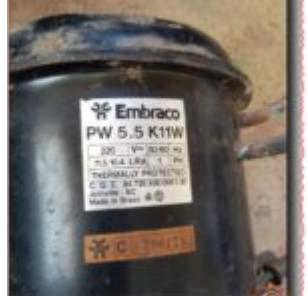
The Embraco PW 5.5 K11W is a 1/6 HP Low Back Pressure (LBP) compressor designed for R12 refrigeration systems. Known for its reliability and dual-frequency 50/60Hz operation, this Brazilian-made unit delivers 133W of cooling capacity. Explore our deep dive into its electrical specifications, performance tables, and comparison with modern HVAC cooling alternatives.
