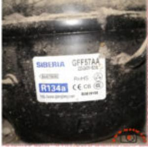
The Siberia GFF57AA is a high-performance 1/5 HP hermetic reciprocating compressor designed for Low Back Pressure (LBP) applications. Utilizing R134a refrigerant and a 5.7cc displacement, it provides a reliable cooling capacity of 166W. This unit is widely used in domestic freezers and refrigerators, offering a robust RSIR motor for 220-240V 50Hz electrical systems.
