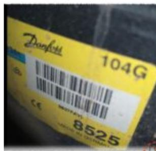
The Danfoss SC15G (104G8525) is a high-capacity 1/2 HP compressor designed for R134a commercial cooling applications. Featuring a 15.28cc displacement and German engineering, it excels in MBP/HBP environments like display coolers. This professional guide details its 738W cooling capacity, electrical requirements, and provides a comprehensive cross-reference list for field technicians and engineers.
