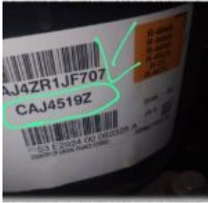
The Tecumseh CAJ4519Z stands as a benchmark in commercial refrigeration, offering robust performance for Medium and High Back Pressure (MHBP) applications. Engineered for versatility, it supports a wide array of refrigerants including R404A and R407C. This professional analysis covers technical data, wiring configurations, and essential maintenance practices for field engineers working on refrigeration units.
