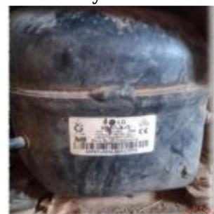
The LG MA57LBJG is a high-performance 1/6 HP compressor designed for R134a refrigerant in Low Back Pressure (LBP) applications. Ideal for domestic freezers, it delivers 160W of cooling capacity at -23.3°C. This guide provides comprehensive technical data, winding details, and a full cross-reference list for professional refrigeration technicians and engineers.
