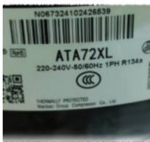
Choosing between the ZEL GQY80AT and Huaguang ATA72XL requires a deep understanding of displacement and cooling wattage. This professional guide breaks down the 198W capacity of the GQY80AT versus the 185W of the ATA72XL, providing essential data for technicians, including oil types, motor configurations, and a comprehensive list of cross-compatible replacement models.
