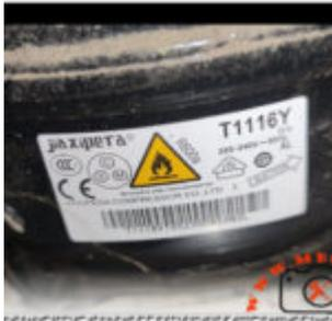
The Jiaxpera T1116Y stands out as a reliable 1/5 HP hermetic piston compressor built for low back pressure (LBP) applications in mini fridges and small freezers. It runs on R600a refrigerant with a 10.5 cm<sup>3</sup> displacement, delivering 184W cooling capacity at -23.3°C.
