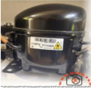
The Jiaxipera TT1114GY is a cornerstone of modern eco-friendly refrigeration, utilizing R600a isobutane to deliver high-efficiency cooling in household appliances. Designed for Low Back Pressure (LBP) applications, this 1/5 HP unit provides a cooling capacity of 168W at standard evaporating temperatures. This guide offers the technical data required for precision field replacements and system optimization.
