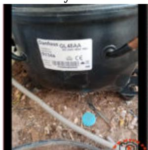
The Danfoss GL45AA is a reliable 1/8 HP R134a compressor designed for low back pressure applications. Used in refrigerators, beverage coolers, and freezers, this thermally protected unit delivers 96 kcal/h cooling capacity at -23.3°C with RSIR motor technology and operates between -35°C to -10°C.
