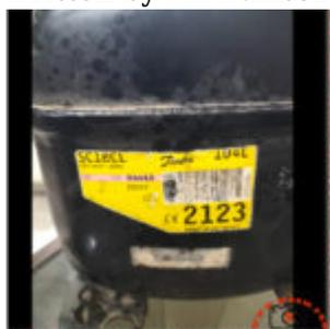
The Danfoss SC18CL compressor (104L2123) is a 5/8 HP hermetic reciprocating compressor designed for commercial refrigeration. Operating on R404A/R507 refrigerants at 220-240V 50Hz, it delivers 781W cooling capacity at -23°C for LBP/MBP applications. This comprehensive guide covers
