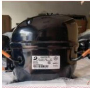
The Donper K400CZ1 is a hermetic reciprocating compressor designed for commercial refrigerators and chest freezers operating with refrigerant R134a on 220-240V 50Hz single-phase power. It offers roughly 1/2 hp class performance with about 400 W cooling capacity, making it suitable for medium-size display cabinets and storage equipment in supermarkets and restaurants.
