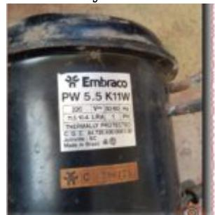
The Embraco PW 5.5 K11W is a 1/6 HP Low Back Pressure (LBP) compressor designed for R12 refrigeration systems. Known for its reliability and dual-frequency 50/60Hz operation, this Brazilian-made unit delivers 133W of cooling capacity. Explore our deep dive into its electrical specifications, performance tables, and comparison with modern HVAC cooling alternatives.
