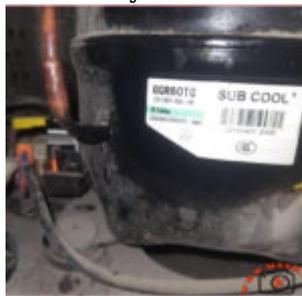
The SUB COOL GQR80TG is a versatile 1/4+ HP compressor designed for R134a MBP/HBP systems, commonly found in commercial coolers and mid-size refrigerators. This guide provides the full technical data sheet, including cooling capacity (400W to 810W depending on conditions), oil requirements (380-420ml POE), and a comprehensive list of compatible replacements for both R134a and modern alternative refrigerants to ensure your repair is successful.
