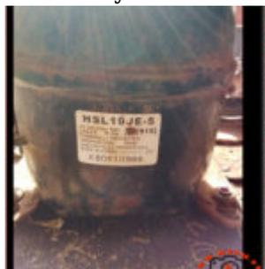
Two workhorse compressors power countless commercial refrigerators and household freezers worldwide. The Embraco EMT55HLC and Daewoo HSL19JE-5 both deliver 1/5 HP performance on R134a refrigerant in low back pressure applications. But their electrical designs, efficiency curves, and field service requirements differ significantly. Here is what technicians need to know.
