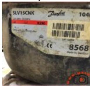
The Danfoss Secop SLV15CNK is a variable-speed LBP hermetic compressor running on R290 propane refrigerant, designed exclusively for commercial freezing applications. With a 15.28 cm<sup>3</sup> displacement, permanent magnet TRI motor, and mandatory SLV electronic controller, it powers chest freezers and display cases across retail worldwide — including AHT deep freezer cabinets.
