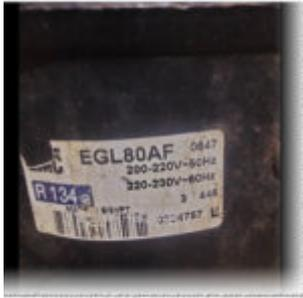
The main difference is the winding material: the GL80 uses aluminum coils, while the GL70 uses copper. Performance-wise, the GL80 is suitable for an upright deep freezer, whereas the GL70 is best for a 12ft double-door refrigerator
