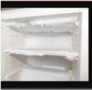
The issues you are experiencing with your Brandt refrigerator (ice buildup, unusual noise, and poor cooling) indicate a failure in the No Frost defrost system. Since a specialist was unable to fix it, the fault may have been misdiagnosed.
