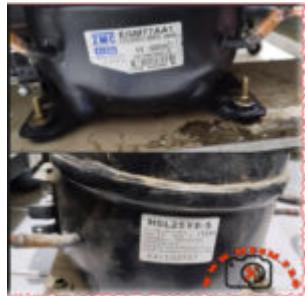
When a refrigerator stops cooling, the heart of the problem is often the compressor. Understanding the differences between the ZMC EGM77AA1 and the Daewoo HSL25YE-5 is vital for any technician. These R134a units are staples in the industry, offering reliable low back pressure performance for domestic and light commercial cooling systems worldwide.
