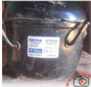
The heart of any reliable industrial or home refrigerator is the compressor. The Siberia GFF93AA stands out as a high-displacement 1/3+ HP unit featuring genuine copper windings and a massive wide-voltage tolerance from 160V to 260V. For technicians working in harsh power zones, this R134a unit provides 270W of efficient, stable cooling power...
