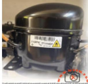
The Jaxipera TT1114GY is a cornerstone of modern eco-friendly refrigeration, utilizing R600a isobutane to deliver high-efficiency cooling in household appliances. Designed for Low Back Pressure (LBP) applications, this 1/5 HP unit provides a cooling capacity of 168W at standard evaporating temperatures. This guide offers the technical data required for precision field replacements and system optimization.
