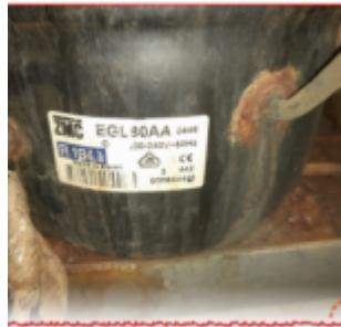
Finding the perfect heart for your 2012 Kiriazi refrigerator requires precision. The ZMC GL80AA 1/5 HP compressor is the definitive OEM standard, offering the perfect balance of cooling capacity and durability for 14ft cabinets. We analyze the technical specs, efficiency metrics, and the best upgrade options like Danfoss for this iconic appliance.
