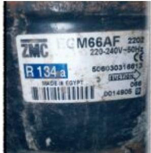
The ZMC EGM66AF is a high-reliability 1/6 HP compressor designed for Low Back Pressure (LBP) applications in domestic refrigerators ranging from 10 to 12 feet. Utilizing R134a refrigerant and a 6.66cc displacement, this unit features durable copper windings and an RSIR motor, making it a preferred choice for technicians seeking longevity and efficiency.
