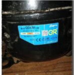
The L55AV and QD59H are cornerstone compressors in the domestic refrigeration industry, both rated at 1/6 HP. While the L55AV traditionally operates with R12, the QD59H is the modern R134a standard. This article provides deep technical data, electrical wiring diagrams, and professional comparison tables for field technicians and refrigeration engineers seeking reliable data.
