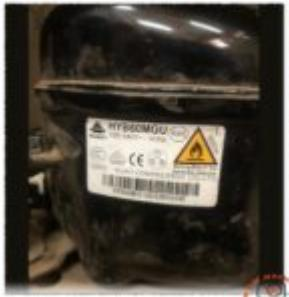
The Huayi HYB60MGU is a high-efficiency hermetic reciprocating compressor specifically engineered for Low Back Pressure (LBP) applications. Operating on the eco-friendly R600a refrigerant, this 1/7 HP unit is a primary component in modern household refrigerators. This guide provides an in-depth technical analysis, electrical wiring configurations, and reliable replacement alternatives for field engineers.
