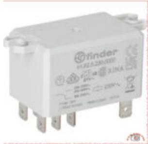
The Finder 66.82.8.230.0000 is a high-power, flange-mount relay designed for demanding switching tasks in HVAC, refrigeration and industrial control panels. With a 230 V AC coil and 30 A contact rating, it offers a compact but robust alternative to contactors in many applications, saving space while maintaining safety.
